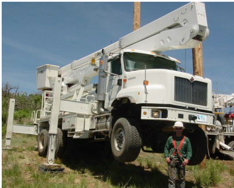
Figure 4. Bucket Truck with Outriggers Down
