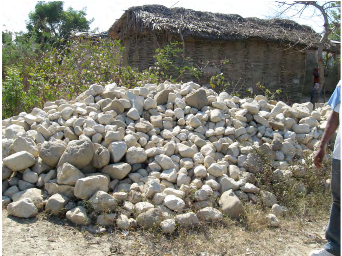
Photograph displaying the significant amount of larger stones needed for a large building's foundation in Haiti
