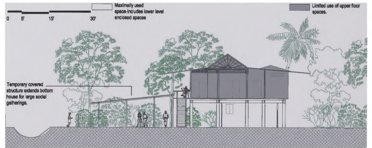
Figure 15b: Sectional Diagram of Jagan House showing Use for a Large Social Gathering
