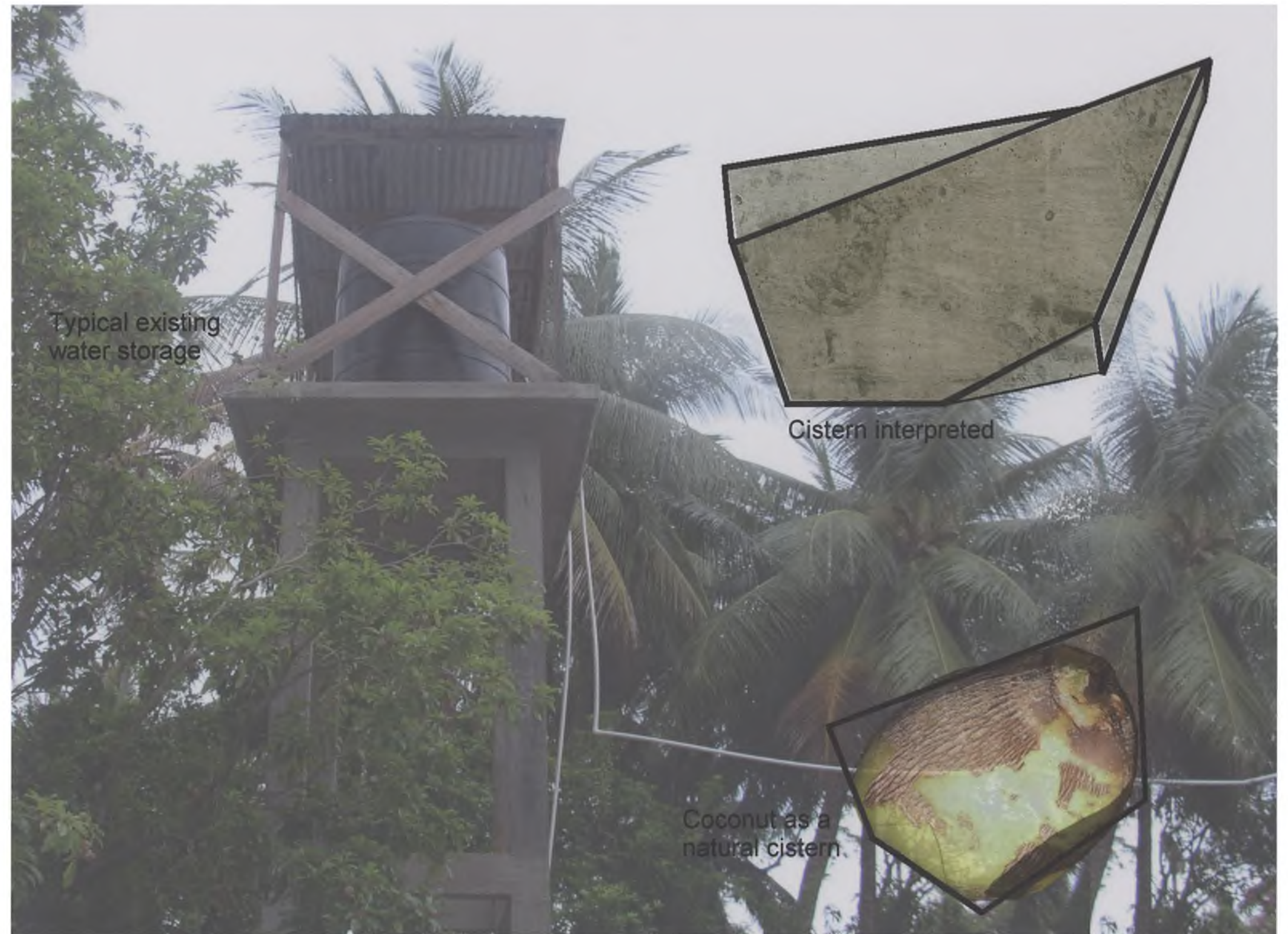
Figure 59: Diagram of Formal Derivation of Water Cistern. The typical existing water cistern in Ankerville is a metal or plastic cylindrical drum placed on a wooden or concrete structure. The Water Cistern for the Women's Center Tower derives its form based upon an analogy of the coconut fruit being a natural cistern. Coconut Palms play a vital role in the daily economic life of most villagers.
